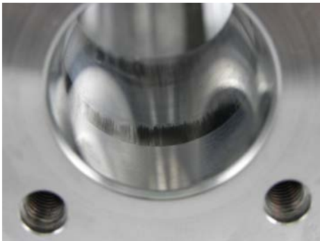
Figure 9 – Post-test SPK Pump Body Bore Polish
