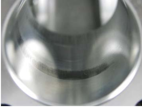
Figure 8 – Post-test ULSD Pump Body Bore Polish
